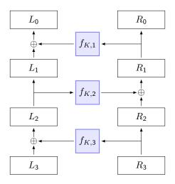
Decryption works backwards ( $i=r,\ldots,1$ ), undoing round after round, starting from the ciphertext:
