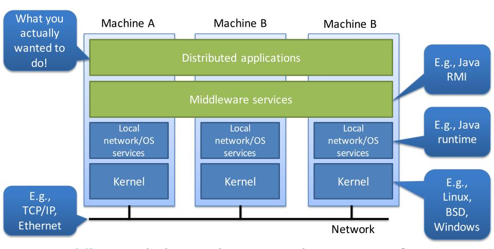
Middleware helps application authors write software intended to run on more than one machine at a time.
