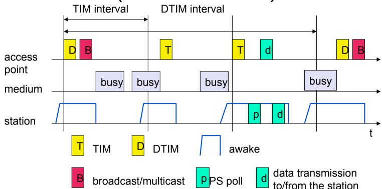
TIM: list of stations for which there will be data in the slot DTIM Interval indicates the delivery traffic indication map: for broadcast and multicast frames. It's a multiple of TIM
