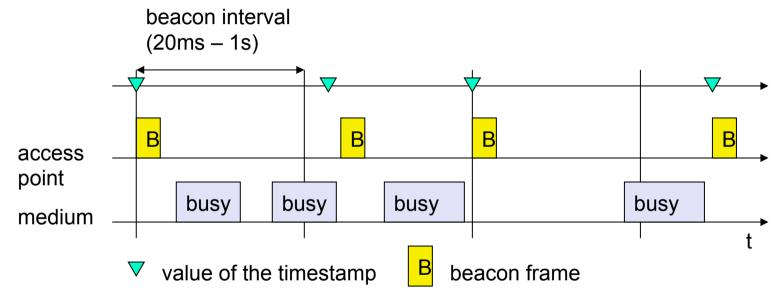
•Nodes need to keep a tight synchronized clock with the access point: this is useful for power management and coordination of frequency hopping or contention slots.
