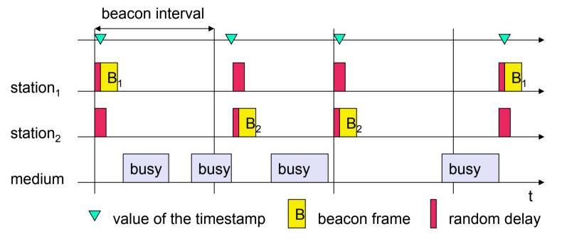
•In ad hoc mode each station transmits a beacon after the beacon interval [semi periodic again]
