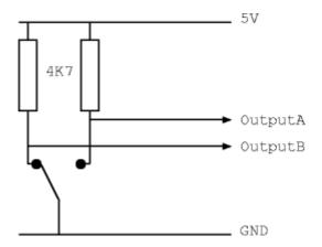
**Task:** Build the above circuit. Design and build a circuit which takes OutputA and OutputB as input and produces a debounced output. Hint: this only requires one latch.
