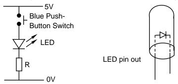
When the LED is lit correctly, the voltage across it will be about 1.6V and the current flowing through it should be about 15mA. To work out the appropriate value for R we need to use Ohm's law, i.e., V = IR. In this case the voltage across R is (5 - 1.6)V, so,
