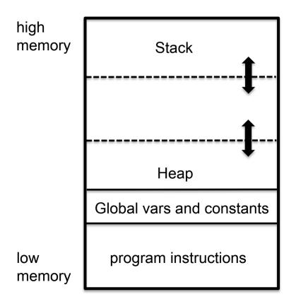
The heap is used for dynamically allocating memory. Typically either for very large objects or for those objects that are returned by functions/procedures and must outlive the associated activation record.
