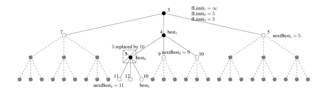
Now  $f(\text{best}_3) > \text{fLimit}_3$  so the function call returns (fail, 10) into (result<sub>3</sub>, f') and  $f(\text{best}_2) = 10$ .
