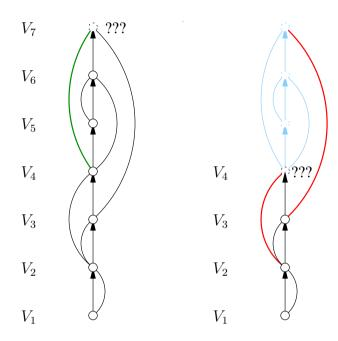
Backjumping from  $V_7$  to  $V_4$  is fine. However we shouldn't then just backjump to  $V_2$ , because changing  $V_3$  could fix the problem at  $V_7$ .
