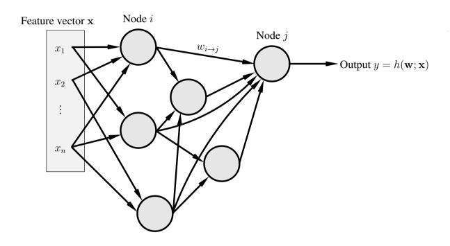
Each node is a perceptron. No specific layering is assumed.  $w_{i\to j}$  connects node i to node j.  $w_0$  for node j is denoted  $w_{0\to j}$ .
