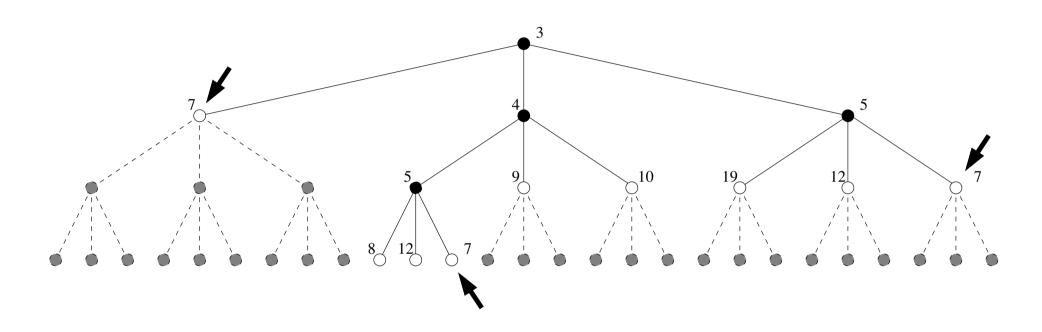
The new limit is 7, so at the next iteration the three arrowed nodes will be explored.
