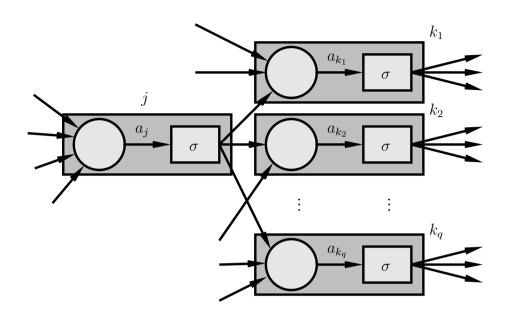
$$\frac{\partial a_k}{\partial a_j} = \frac{\partial}{\partial a_j} \left( \sum_i w_{i \to k} \sigma(a_i) \right) = w_{j \to k} \sigma'(a_j)$$
