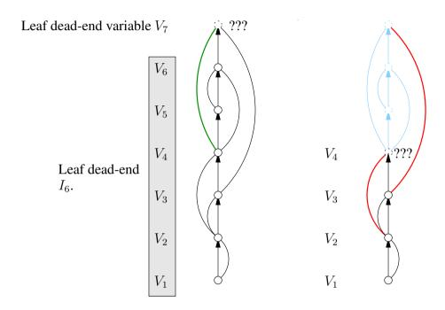
Given an instantiation  $I_k$  and  $V_{k+1}$ , if there is no consistent  $d \in D_{k+1}$  we call  $I_k$  a leaf dead-end and  $V_{k+1}$  a leaf dead-end variable.
