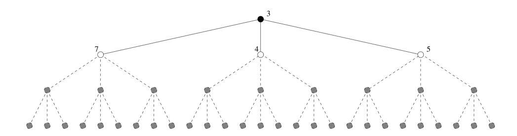
Initially, the algorithm looks ahead and finds the *smallest* f cost that is *greater* than its current f cost limit. The new limit is 4.
