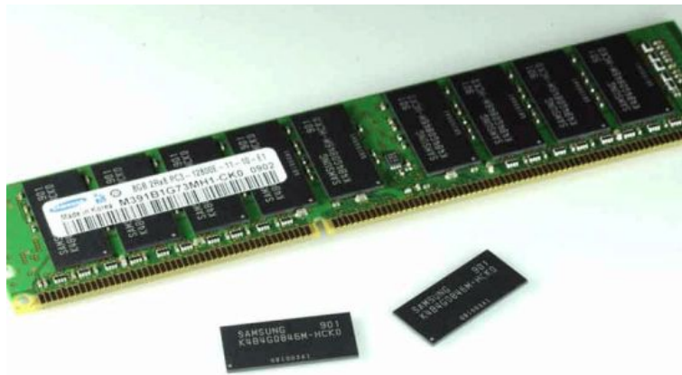
Figure 3.31: DRAM single-in-line memory module (SIMM).
