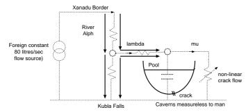
This drawing may suggest the water from the channel spills into the pool. But such an arrangement would be like the Kubla Falls and the flow rate would be unaffected by the current depth. In reality the channel joins the pool below the waterline, and hence backpressure applies.
