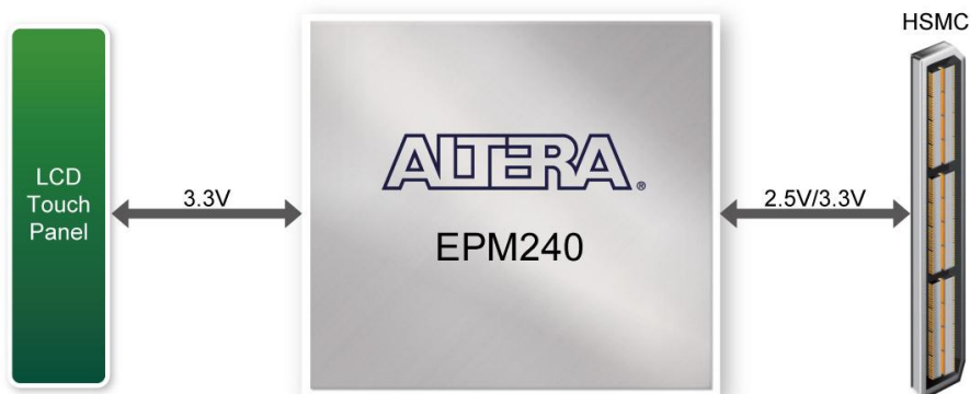
Figure 3-6 Block Diagram of the Bus Controller
