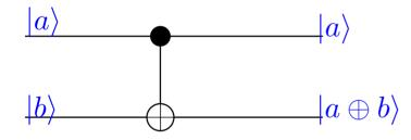
The controlled not flips the second qubit if the first qubit is  $|1\rangle$ and leaves it unchanged if it's  $|0\rangle$
