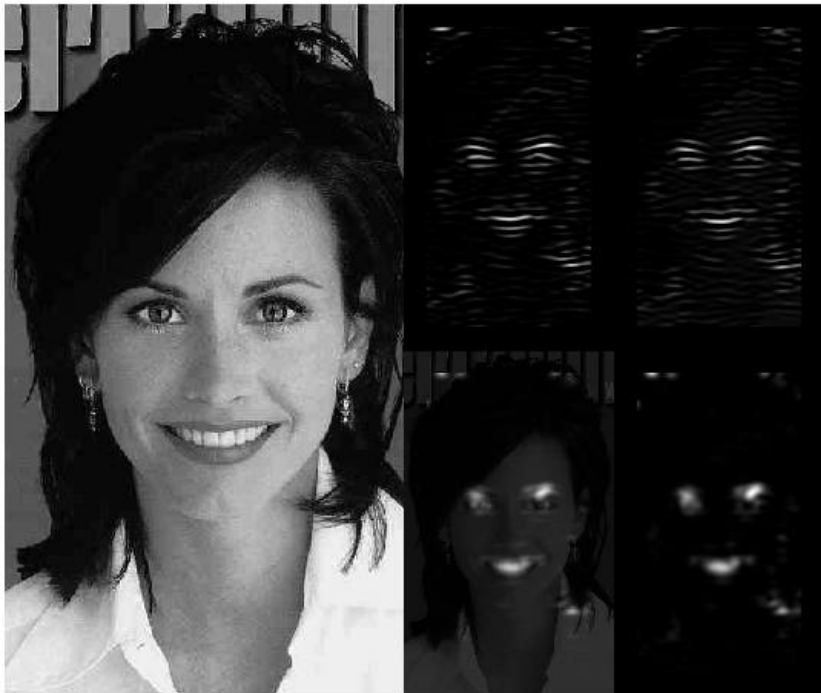
Illustration of Facial Feature Detection by Quadrature Filter Energy. Left panel: original image. Right panel (clockwise from top left): the real part after 2D Gabor wavelet convolution; the imaginary part; the modulus; and modulus superimposed on the original (faint) image, illustrating successful feature localisation by the Quadrature Demodulator Network in the previous Figure.
