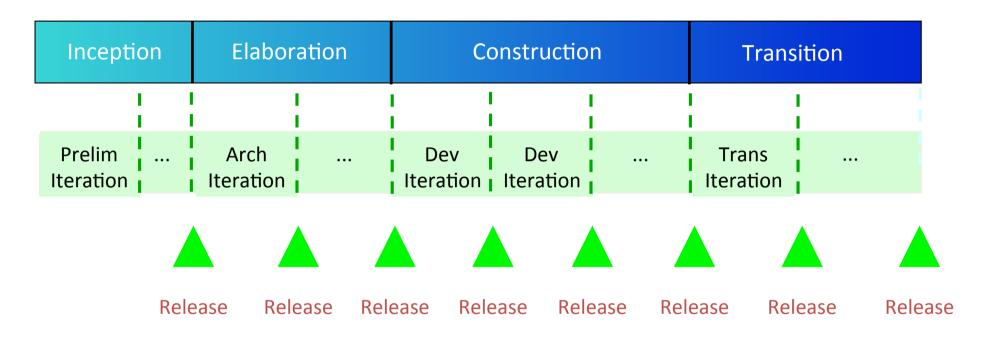
An iteration is a sequence of activities with an established plan & evaluation criteria, resulting in an executable release
