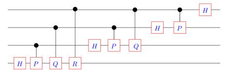
In the input, the least significant bit is at the top, in the output, it is at the bottom.
