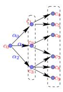
The machine can be seen as progressing through a series of stages, each of which is a superposition of configurations.
