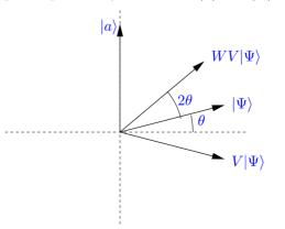
V is a reflection about the line perpendicular to  $|a\rangle$ . W is a reflection about  $|\Psi\rangle$ . The composition of two reflections of the
