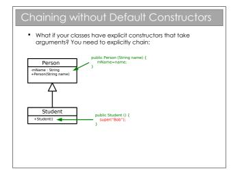
This can get messy though: what if the parent does not have a default constructor? In this case, the code won't compile, and we will have to manually add a call to **super** ourselves, using the appropriate arguments.
