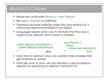
Abstract classes allow us to partially define a type. Because it's not fully defined, you can't make an object from an abstract class (try it). Only once all of the 'blanks' have been filled in can we create an object from it. This is particularly useful when we want to represent high level concepts that do not exist in isolation.
