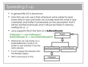
The reason file I/O is typically so slow is that hard drives take a long time to deliver information. They contain big, spinning disks and the read head has to move to the correct place to read the data from, then wait until the disc has spun around enough to read all the data it wanted (think old 12 inch record players). Contrast this with memory (in the
