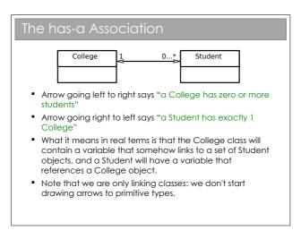
The graphical notation used here is part of UML (Unified Modeling Language). UML is a standardised set of diagrams that can be used to describe software independently of any programming language used to implement it.
