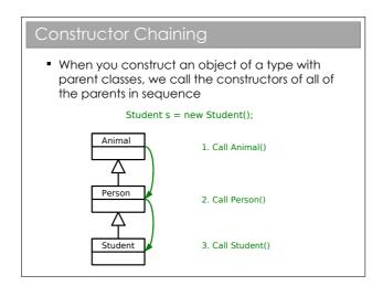
What actually happens is that the first line of a constructor *always* starts with super(), which is a call to the parent constructor (which
