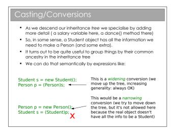
One way to think about this is that when we create a new Student the computer allocates a chunk of memory for that object. In that chunk there is space for all of the fields (name, age, exam score, etc) and definitions of the methods it supports. Because a Student is a Person, that chunk will contain everything required for a Person (name, age) and some extras specific to being a Student (exam score).
