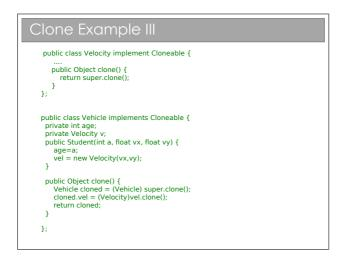
A deep clone requires that we clone the objects that are referenced (and they, in turn clone any objects they reference, and so on). Here we make Velocity cloneable and make sure to clone the member variable that Vehicle has.
