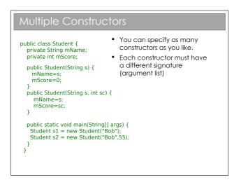
**Beware:** As soon as you specify *any* constructor whatsoever (regardless of the arguments), no default constructor will be generated. The default constructor only applies when the compiler notices that there is no way to construct an object of this type, which can't be intentional or what's the point of writing the class?
