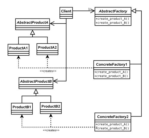
Note that usually there is no need to make more than one factory for a given family, so we can use the **Singleton** pattern to save memory and time.
