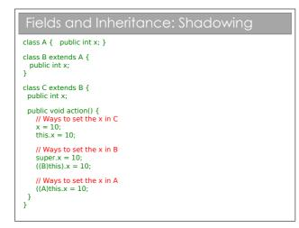
What happens here?? There is an inheritance tree (A is the parent of B is the parent of C). Each of these declares an integer field with the name x.
