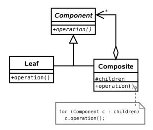
Notice the terminology in the general case: we speak of **Lea**fs because we can use the Composite pattern to build a *tree* structure. Each **Composite** object will represent a node in the tree, with children that are either **Composite**s or **Lea**fs.
