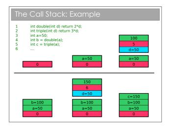
In this example I've avoided going down to assembly code and just assumed that the return address can be the code line number. This causes a small problem with e.g. line 4, which would be a couple of machine instructions (one to get the value of double{) and one to store it in b). I've just assumed the computer magically "remembers" to store the return value here for brevity.
