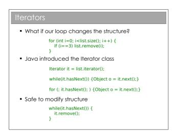
Note that the foreach structure isn't useful with **lterators**. So we sacrifice some code readability for the ability to adjust the **Collection**'s structure as we go.
