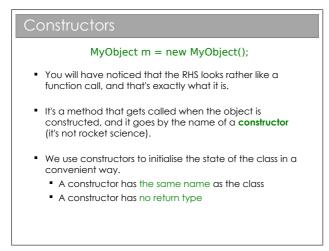
You can't specify a return type for a constructor because it is always called using the special **new** keyword, which must return a reference to the newly constructed object. You can, however, specify arguments for a constructor in the same way as usual for a method.
