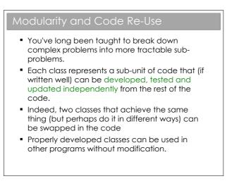
Modularity is extremely important in OOP. It's the usual CS trick: break big problems down into chunks and solve each chunk. In this case, we have large programs, meaning scope for lots of coding bugs. By identifying objects in our problem, we can write classes that represent them. Each class can be developed, tested and maintained independently of the others (assuming we've done a good job).
