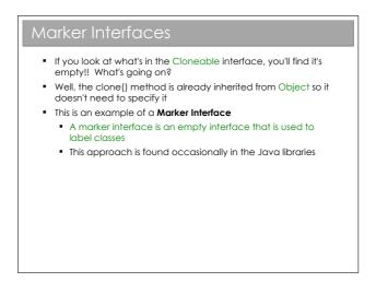
You might also see these marker interfaces referred to as *tag interfaces*. They are simply a way to label or tag a class. They can be very useful, but equally they can be a pain (you can't dynamically tag a class, nor can you prevent a tag being inherited by all subclasses).
