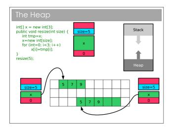
For those who did the Paper 2 O/S course, you should realise that the heap gets *fragmented*: as we create and delete stuff we leave holes in memory. Occasionally we have to spend time 'compacting' the holes (i.e. shifting all the stuff on the heap so that it's used more efficiently.
