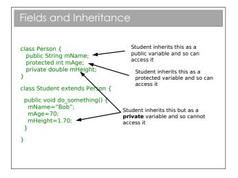
You will see that the **protected** access modifier can now be explained. A **protected** variable is exposed for read and write within a class, and *within* all subclasses of that class. Code outside the class or its subclasses can't touch it directly<sup>1</sup>.
