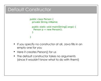
*Every* class has a constructor. The only question is whether it's been specified manually by the programmer or whether the compiler has filled in a default (empty) constructor.
