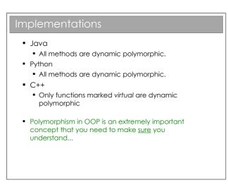
C++ allows you to choose whether methods are inherited statically (default) or dynamically (explicitly labelled with the keyword 'virtual'). This can be good for performance (only incur the overhead when you need to), but gets complicated, especially if the base method isn't dynamic but a derived method is...
