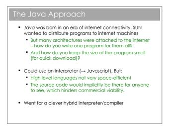
Sun Microsystems invented Java as the web started to take off. Suddenly many different devices with many different machine architectures were communicating and they wanted to produce programs that could be run on any machine. They could have sent source code to an interpreter in the browser (a valid approach - it's what javascript does), but they i) wanted to get the best performance they could and ii) realised that there are times when you want to distribute binary files not source code.
