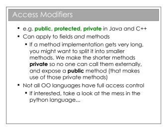
At this stage you should be comfortable with public and private fields of a class. The former allows code outside of the object to read it and alter it; whilst the latter prevents any access to the field from outside the class. protected we will come to shortly....
