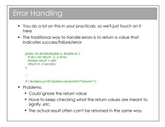
In some cases the range of potential results is smaller than the range of return values, in which case we can use the 'spare' values to signify error. E.g. If we know the result will be positive, we can use -1 to signify an error. Whilst this works (and is extremely common in C), it means that we have to write 10 or more lines of error checking code for every line of meaningful program!
