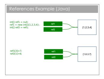
In this example, we create a reference and set it to null. Then we create a new array (using the new keyword and assign the reference to point to it. Then we create another reference with the same value as ref1. i.e. we have two references pointing to the same array in memory.
