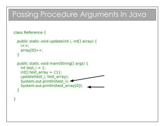
This example is taken from your practicals , where you observe the different behaviour of test\_i and test\_array—the former being a primitive int and the latter being a reference to an array.
