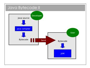
So Java is a bit of a half-way house. It compiles high-level source code into binary files that use a special instruction set called **bytecode**. You can think of this as being machine code for a virtual, generic CPU. Ironically there are now CPUs that use the bytecode instruction set but that wasn't really the intention.
