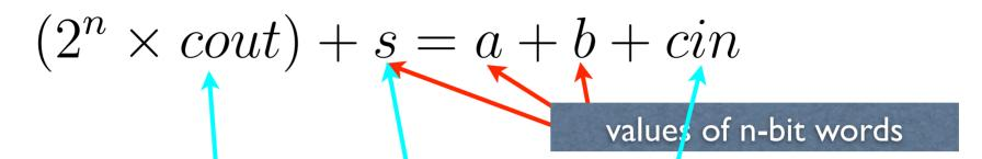
The function bits\_val converts a binary numeral (supplied in the form of a boolean valued function, f) to a non-negative integer. The specification of the adder then follows the obvious arithmetic specification closely. When n=0, the specification merely requires cin=cout.
