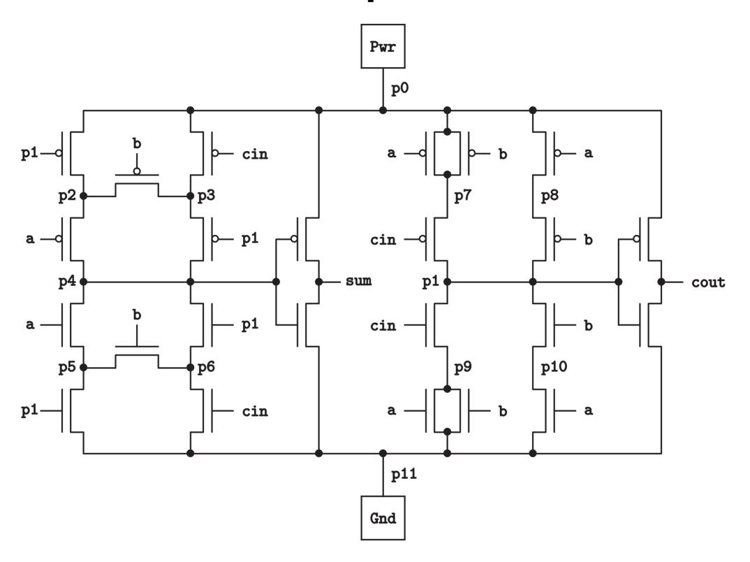
A full adder is easily expressed at the gate level in terms of exclusive-OR (to compute the sum) and other simple gating to compute the carry. The diagram above, again from Prof Gordon's notes, expresses a full adder as would be implemented directly in terms of transistors.
