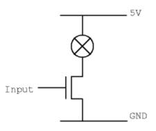
**Task 4**: Replace the output filter with a light bulb and driver transistor as shown below. Since the temperature of the light bulb filament has inertia, it provides a filtering effect on the light output. Answer question 9.
