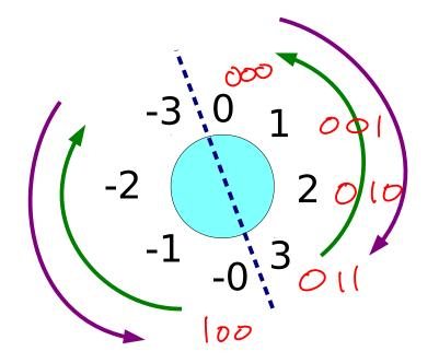
Gives us two discontinuities and a reversal of direction using normal addition circuitry!!
