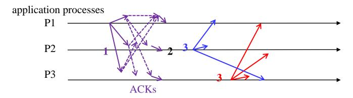
P1 increments its clock to 1 and multicasts a message with timestamp 1 All delivery systems collect the message, multicast ACK and collect all ACKs - no contention – deliver message to application processes and increment local clocks to 2.
