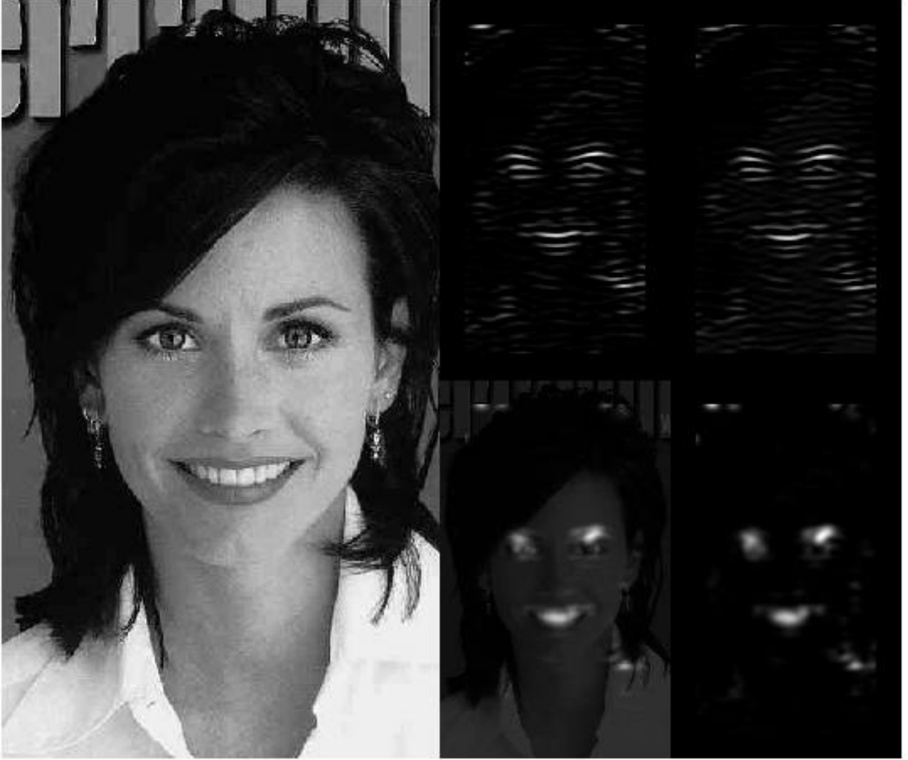
Illustration of Facial Feature Detection by Quadrature Filter Energy. Left panel: original image. Right panel (clockwise from top left): the real part after 2D Gabor wavelet convolution; the imaginary part; the modulus; and modulus superimposed on the original (faint) image, illustrating successful feature localisation by the Quadrature Demodulator Network in the previous Figure.
