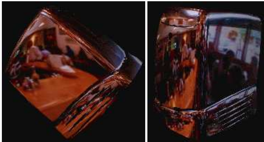
Figure 8: An example of environment mapping: a silvered SGI O2 computer reflecting an environment map of the interior of a cafe.
