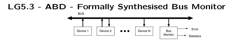
A bus monitor connects to the net-level bus.
