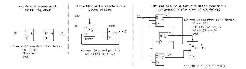
Two implementations of a two-bit shift register.
