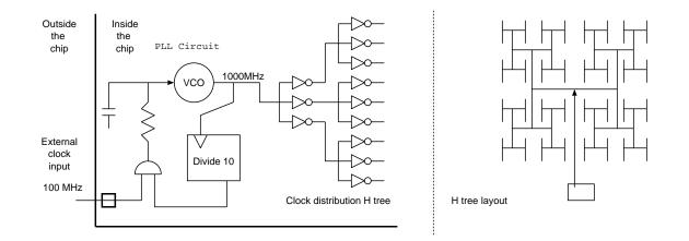
Clock sourced from a lower-frequency external (quartz) reference.
