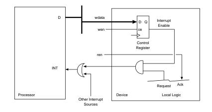
Receiving device: Keep int enabled: dev interrupts when data ready.
