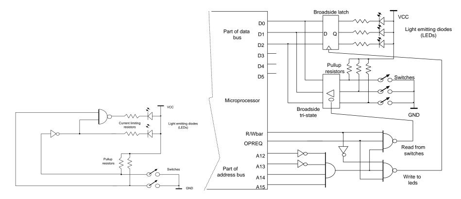
a) Example of electronic wiring for switches and LEDs.
