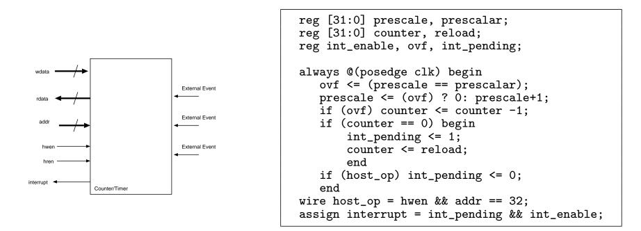
Re-load register accommodates poor interrupt latency.
