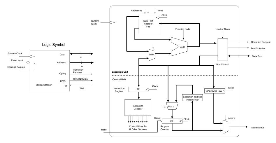
A microprocessor logic symbol and simplified internal structure.
