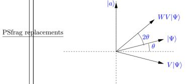
V is a reflection about the line perpendicular to  $|a\rangle$ . W is a reflection about  $|\Psi\rangle$ . The composition of
