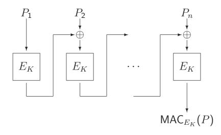
A modification of CBC provides integrity protection for data. The initial vector is set to a fixed value (e.g., 0), and  $C_n$  of the CBC calculation is attached to the transmitted plaintext. Anyone who shares the secret key K with the sender can recalculate the MAC over the received message and compare the result. A MAC is the cryptographically secure equivalent of a checksum, which only those who know K can generate and verify.
