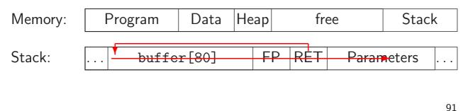
Overwriting the return address is the most common form of a buffer overflow attack. If the return address cannot be reached, alternatives include:
