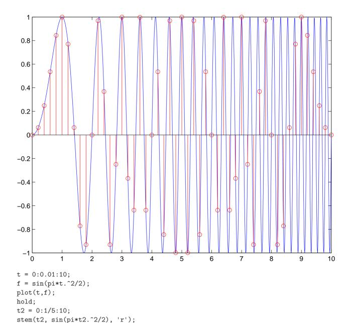
(d) A sine wave with a frequency f larger than half the sampling frequency  $f_s$  cannot be distinguished based on the sample values from a sine wave of frequency  $f_s - f$ . In other words, the sample values would have looked the same had we replaced the instantaneous frequency f(t) with  $f_s/2 - |f_s/2 - f(t)|$ , and the latter is symmetric around  $f_s/2$ , which is in this graph 2.5 Hz and occurs at t = 5 s.
