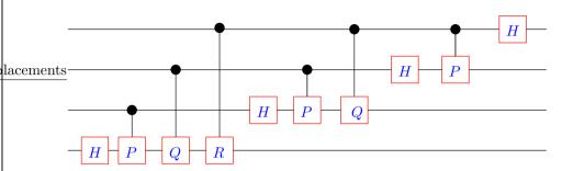
In the input, the least significant bit is at the top, in the output, it is at the bottom.
