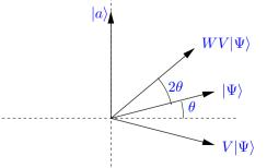
V is a reflection about the line perpendicular to  $|a\rangle$ . W is a reflection about  $|\Psi\rangle$ . The composition of two reflections of the plane is always a rotation.
