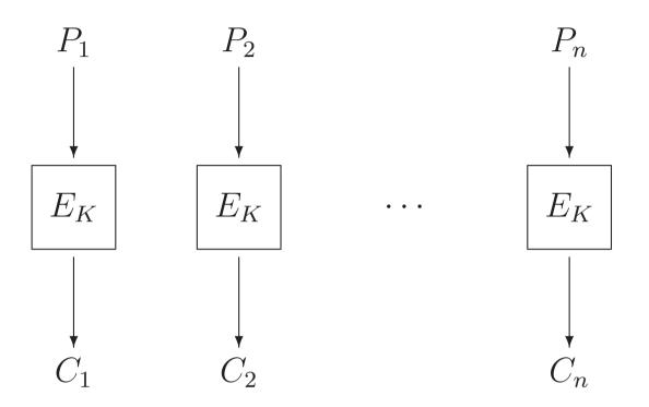
In the simplest **mode of operation** standardised for DES, AES, and other block ciphers, the message is cut into n-bit blocks, where n is the block size of the cipher, and then the cipher function is applied to each block individually.
