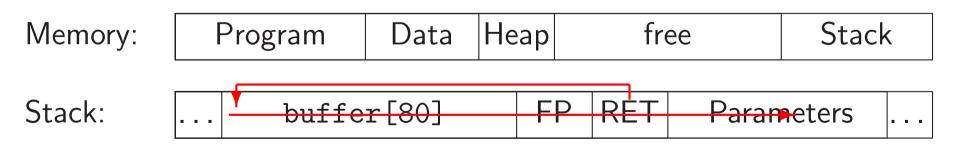
Overwriting the return address is the most common form of a buffer overflow attack. If the return address cannot be reached, alternatives include:
