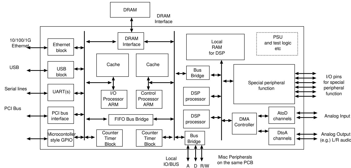
System on a Chip = SoC design.
