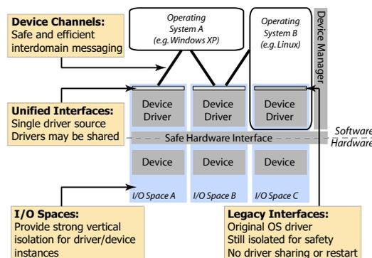
Figure 1: Design of the safe hardware model.
