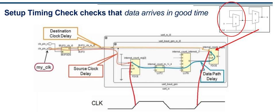
Checks that change in a clocked element has time to propagate to other clocked elements before the next clock event
