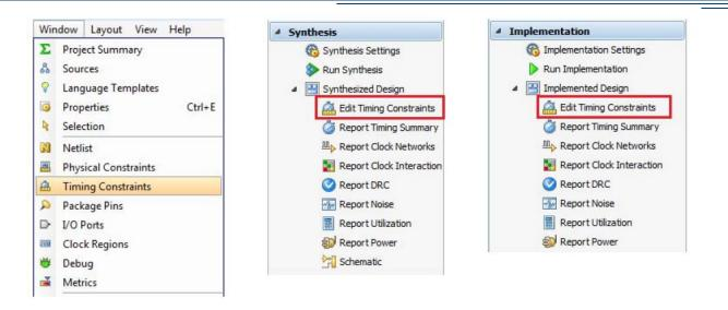
Constraints include: **Timing constraints**, Pin assignments, Placement constraints (floorplanning), Properties and Attributes.
