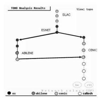
Fig. 6. Graphical traceroute display. Note hop to ABILENE on the way to CENIC
