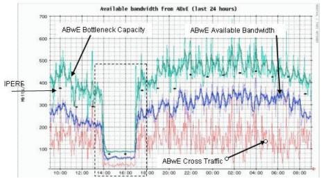
**Fig. 4.** Plot of ABwE (available bandwidth) measurements and corresponding IPERF (achievable bandwidth) measurements
