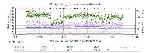
**Fig. 1.** Time series plot with route changes indicated. The asterisks along the top axis indicate the forward traceroute changes. The asterisks along the bottom axis indicate reverse route changes. Note the correspondence between throughput changes and forward route changes
