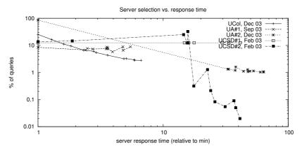
**Fig. 1.** Distributions of queries among root servers vs. response time. Each point on the plots shows percentage of queries sent to a given root server; the points are plotted in order of increasing response time.
