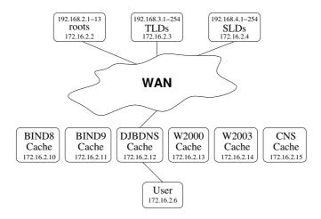
**Fig. 3.** Network setup for DNS tests. The "User" system sends DNS queries to only one of the caches in each test. The cache recursively resolves queries for the user by talking to the authoritative root, TLD, and SLD servers. For some tests we introduce wide-area packet loss and transmission delays with FreeBSD's dummynet.
