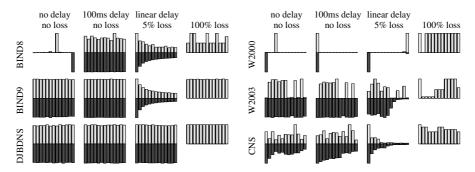
**Table 5.** Distribution of queries to root and *com* TLD nameservers, showing how the caching nameserver distributed its queries in each test. The upper, lighter bars show the histogram for root nameservers. The lower, darker bars show the histogram for the *com* TLD nameservers.
