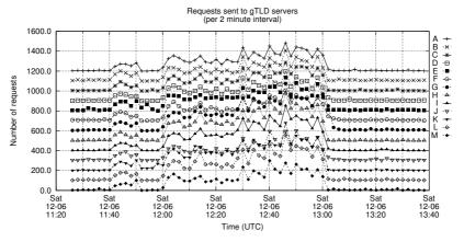
**Fig. 2.** Query rates to gTLD servers. Each subsequent plot is shifted up by 100. There were two periods of connectivity loss when no answers were received: from 11:40 till 11:50 and from 12:00 till 13:00. During these periods query rates increased considerably.
