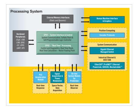
Zynq-7000 EPP devices offer a unique blend of performance and flexibility to meet the high-processing demands and integration required for current and future motor control systems.
