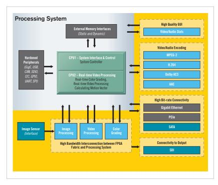
Zynq-7000 EPP devices provide very high bit-rate bandwidth for high-accuracy video processing and analytics in broadcast-level camera systems.
