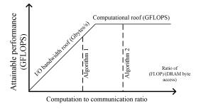
Figure 3: Basis of the roofline model
