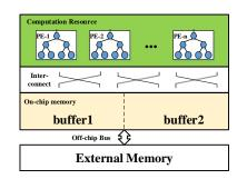
Figure 4: Overview of accelerator design
