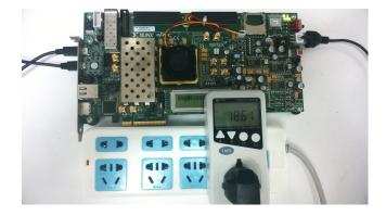
Figure 14: Power measurement of on-board execution
