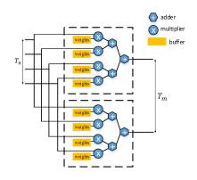
Figure 7: Computation engine
