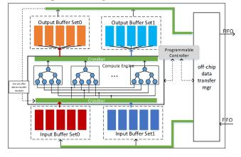
Figure 11: Block diagram of proposed accelerator
