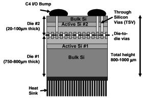
Figure 9: Three dimensional interconnect with stacking
