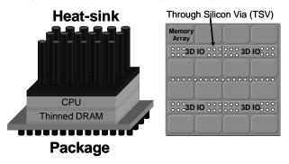
Figure 10: Assembly of 3D memory
