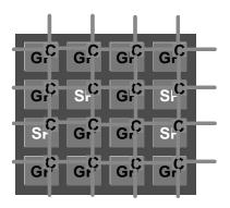
Figure 4: Illustration of a Many Core System
