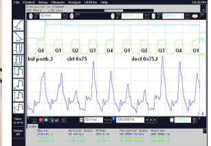
Fig.4. SPA results for PIC16F628
