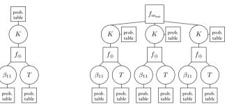
Factor graphs for single (left) and multiple encryptions (right)
