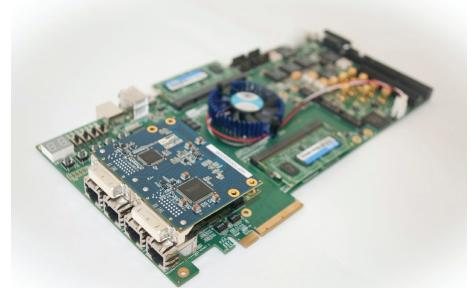
CHERI's 64-bit MIPS-derived CPU prototype, like the BERI prototyping platform it is built on, is written in the **Bluespec hardware description** language (HDL), which facilitates rapid prototyping and design space exploration. The starting point for our hybrid software
