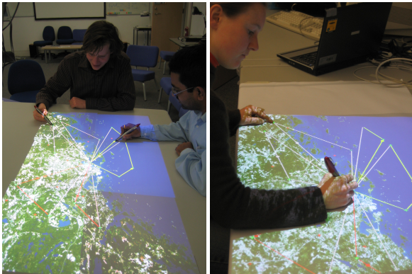
Figure 7: Mixed-presence command and control interfaces using T3. Two co-located participants (left) collaborate with a remote participant (right).
