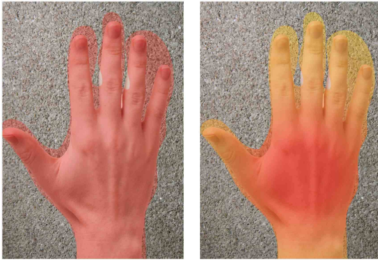
Figure 3.3: Left: a simplification of the original Crayons interface, which shows pixel classification based on a binary threshold. Right: confidence-based colouring exposes how the classifier may still be uncertain about the fingers, and additional annotation may be beneficial.
