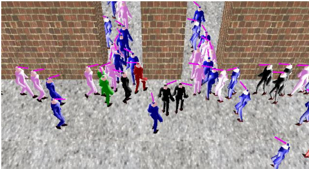
Figure 6.14: Actors evacuating through two narrow doors
