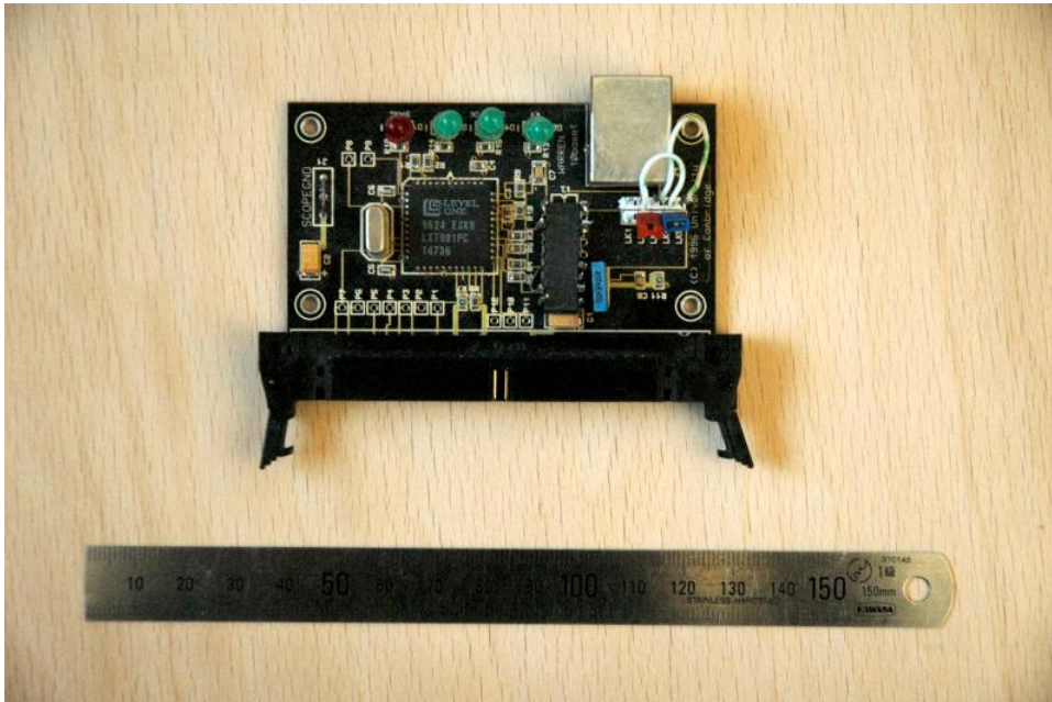
Figure 4.3: Warren PCB showing Intel LXT901
