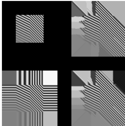
Figure 4.22: How the edge extension methods cope with a pathological case. At top left is the original which consists of diagonal lines at 22.5^\circ (left half) and 45^\circ (right half). Bottom left is extrapolated by copying, this fails for either case as it extrapolates horizontally or vertically. Top right is White and Brzakovic's [1990] derivative method (figure 4.10), and bottom right is our modification of that method (figure 4.11). Both of these perform excellent extrapolation of the 45^\circ features, but fail for the 22.5^\circ features, extending them horizontally, vertically, or at 45^\circ .
