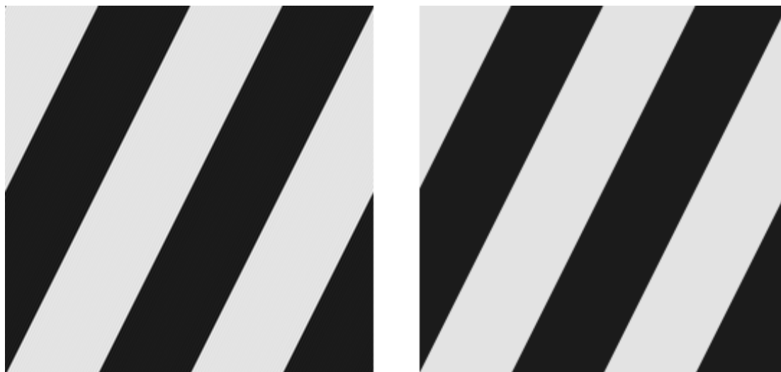
Figure 2.10: Two very similar images: (a) on the left, was generated by summing the first twenty-nine terms of the Fourier series representation of the appropriate square wave; (b) on the right, was generated by super-sampling a perfect representation of the stripes.
