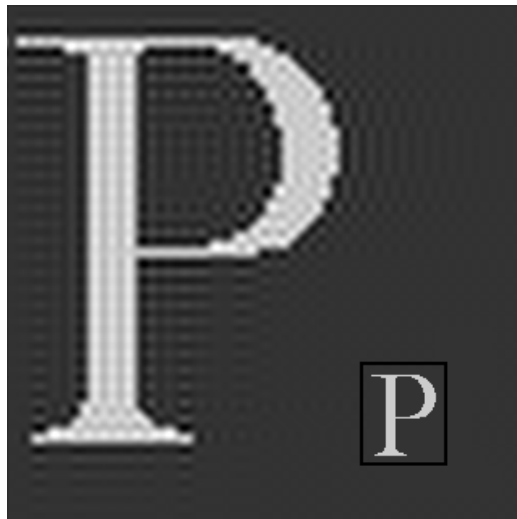
Figure 2.8: An example of a reconstructed intensity surface which contains aliases. These manifest themselves as ripples around the sharp edges in the image. The small image of the letter 'P' is the original. The large is an intensity surface reconstructed from this small original using an approximation to sinc reconstruction.
