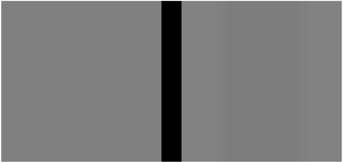
Figure D.3: Two intensity curves which produce roughly the same response from the human visual system. The profiles of the 'edges' in the two images are shown in figure D.2(c) and (d) (left and right images respectively). The left hand image has no edges, while the right has slowly changing edges one quarter and three quarters of the way across the image. Thus, in the right hand image, the intensity at the centre of the image is not the same as the intensity at the left and right edges, even though it looks virtually the same. (After Cornsweet [1970] fig 11.3).
