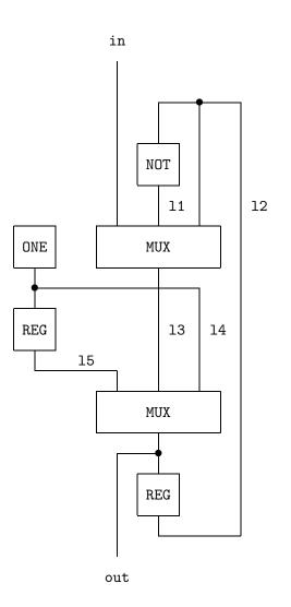
The devices making up this schematic will be modelled with predicates [4]. For example, the predicate ONE is true of a signal out if for all times t the value of out is T.
