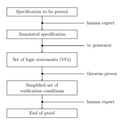
The system takes as input a partial correctness specification annotated with mathematical statements describing relationships between variables. From the annotated specification the system generates a set of purely mathematical statements, called *verification conditions* (or VCs). In Section 3.5 it is shown that if these verification conditions are provable, then the original specification can be deduced from the axioms and rules of Hoare logic.
