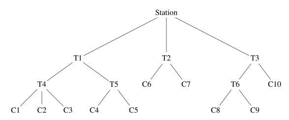
Nodes C1 to C10 are consumers; nodes T1 to T6 are transformers. Each consumer has a direct connection to only one transformer. Sometimes a transformer may malfunction or need to be taken out of service temporarily.
