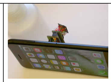
Fig.9. iPhone 7 with NAND wired to connector
