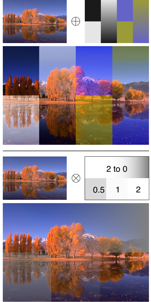
Figure 2: Isomorphic image processing: color shift by color addition \oplus and contrast change by scalar multiplication \otimes .
