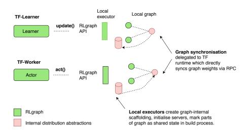
Figure 3.12: Graph-internal and graph-external distributed coordination.
