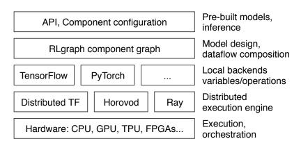
Figure 3.3: RLgraph software stack.
