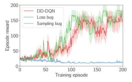
Figure 3.13: DQN training results with bug-free implementation, loss-fault injection, and sampling fault-injection.
