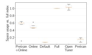
Figure 6.3: Index sizes of the created indices in the fixed blackbox setting with fixed weight initialisation.
