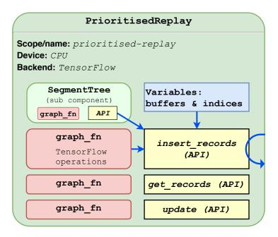
Figure 3.4: Example memory component with three API methods.
