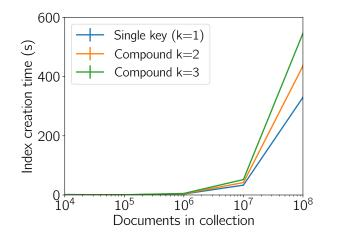
Figure 5.3: Index creation times as a function of document size and the number of attributes k spanned by an index.
