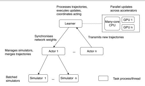
Figure 3.2: High-level overview of single-learner task parallelism. Even in single learner scenarios, multiple levels of task-parallelism require fine-tuning of a multitude of hyper-parameters for distributed coordination.
