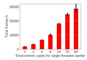
Figure 3.1: Environment vectorisation on CartPole. A single-threaded worker vectorises action selection, then sequentially acts on a list of simulator copies.
