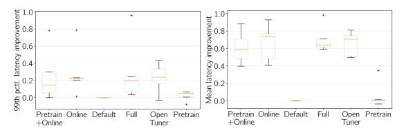
Figure 6.8: 99th percentile (left) and mean (right) relative latency improvements against unindexed configuration in the randomised generalisation task.
